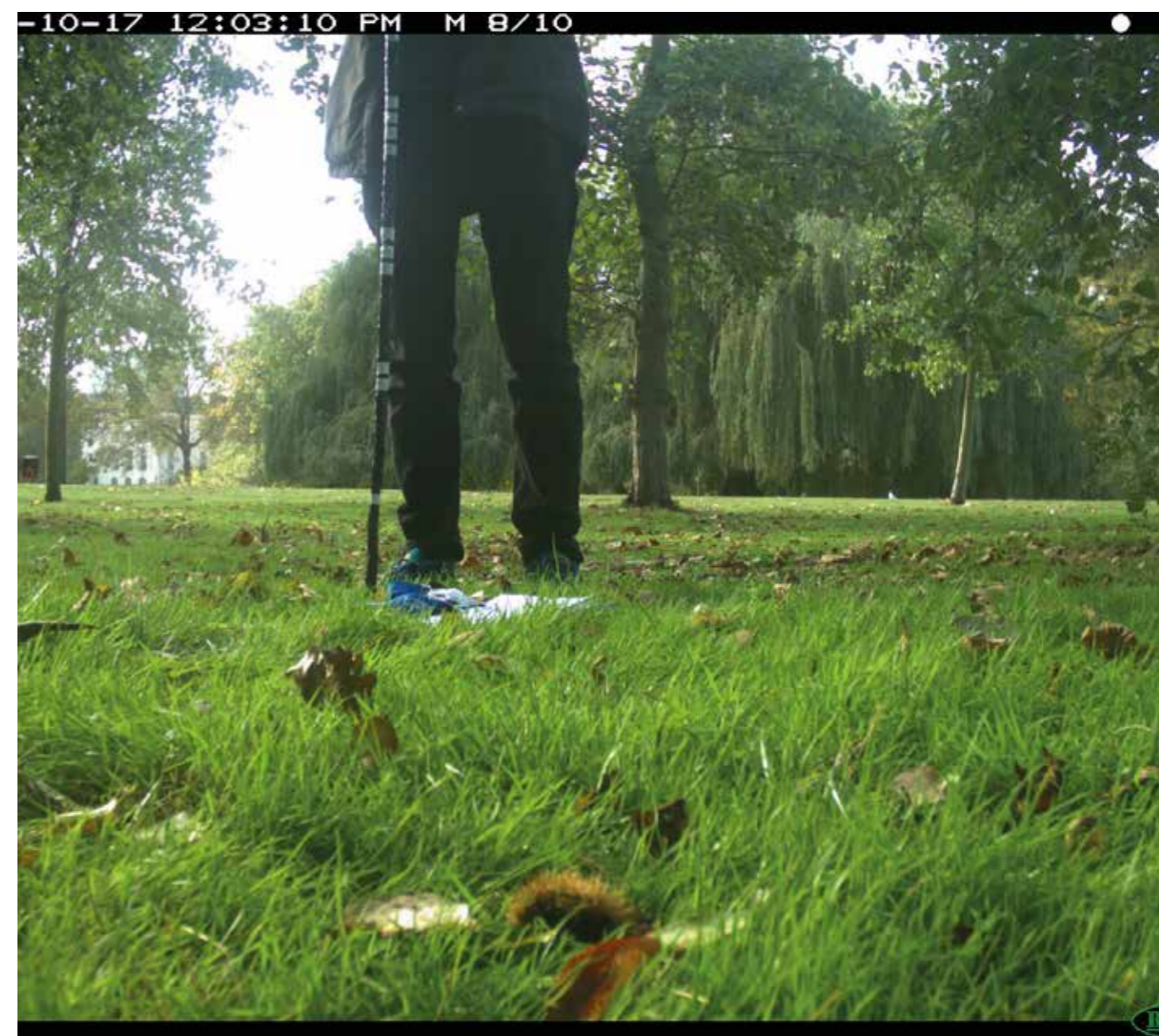
▲ Figure 3. Camera trap image showing the calibration process, a straight pole with markings every 20 cm for building a 3D depth map used in the random encounter model for estimating density. (© Zoological Society London)
