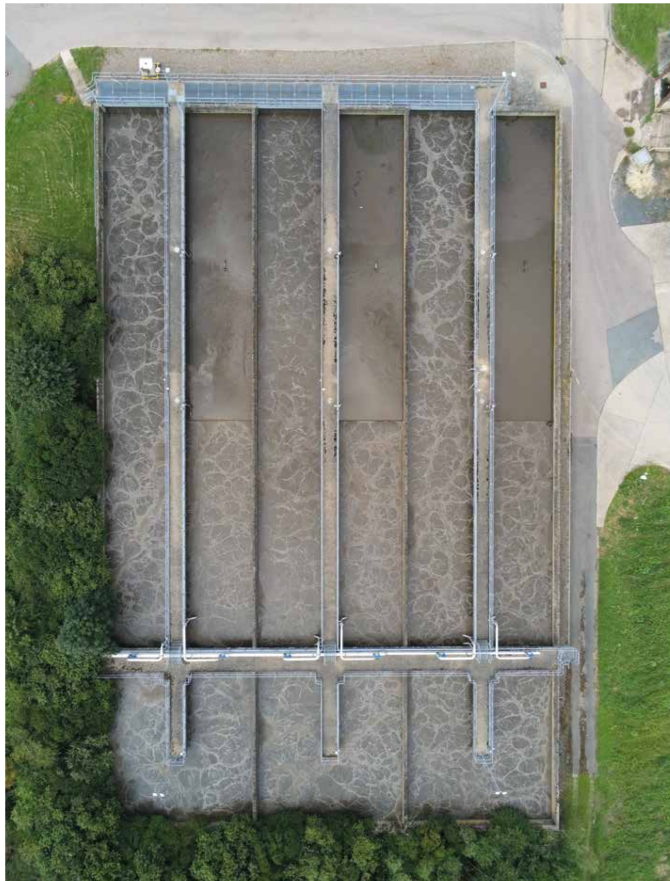
▲ Figure 2. High-resolution imagery of an activated sludge facility using an unoccupied aerial vehicle. (© Severn Trent Water)
